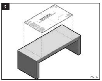
5. Slide The bench over the coach bolts and tighten. Position drilling template as you would the stove.
